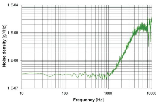
The SM1500 accelerometer is based on a variable capacitor transducer and a feedback circuit that operates in a closed-loop configuration. The feedback force is controlled by an application-specific integrated circuit (ASIC) which provides high reliability and low output noise.
